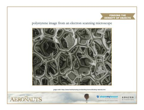
Additionally, as part of the Styrofoam manufacturing process, polystyrene is expanded with air. As a result the molecules are not as tightly packed and there is empty space. Here is a picture of polystyrene foam from an electron scanning microscope.
