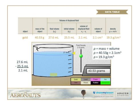
To fill out the data table, we will find the mass of the objects using the digital balance. We will find the volume of the objects using displacement. Then we will calculate the density.
