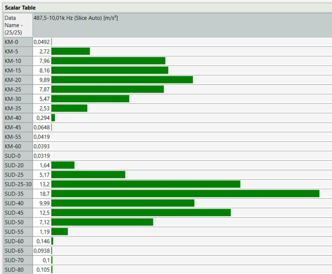
Fig. 3. Distribution of the total RMS in the 500-10000 Hz range corresponding % opening of each valve
