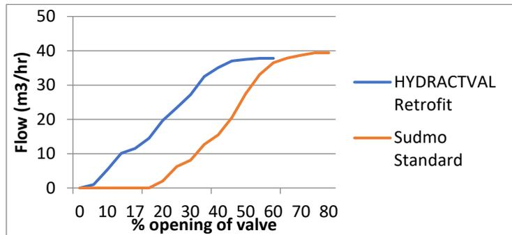
Fig. 1. Flow characteristic comparison
