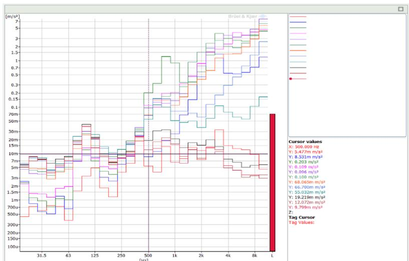
Fig. 2. Vibration spectra on Hydract valve in range 0 to 60% open (1/3 Octave spectra)
