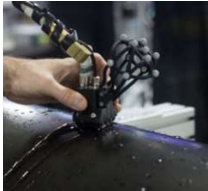
Figure 3. Detail of ergonomic implementation of the IR markers on the UT module.
