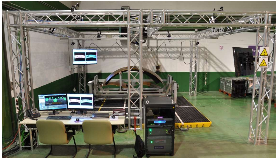
Figure 2. Industrial implementation of an inspection cell based on IR visual tracking.
