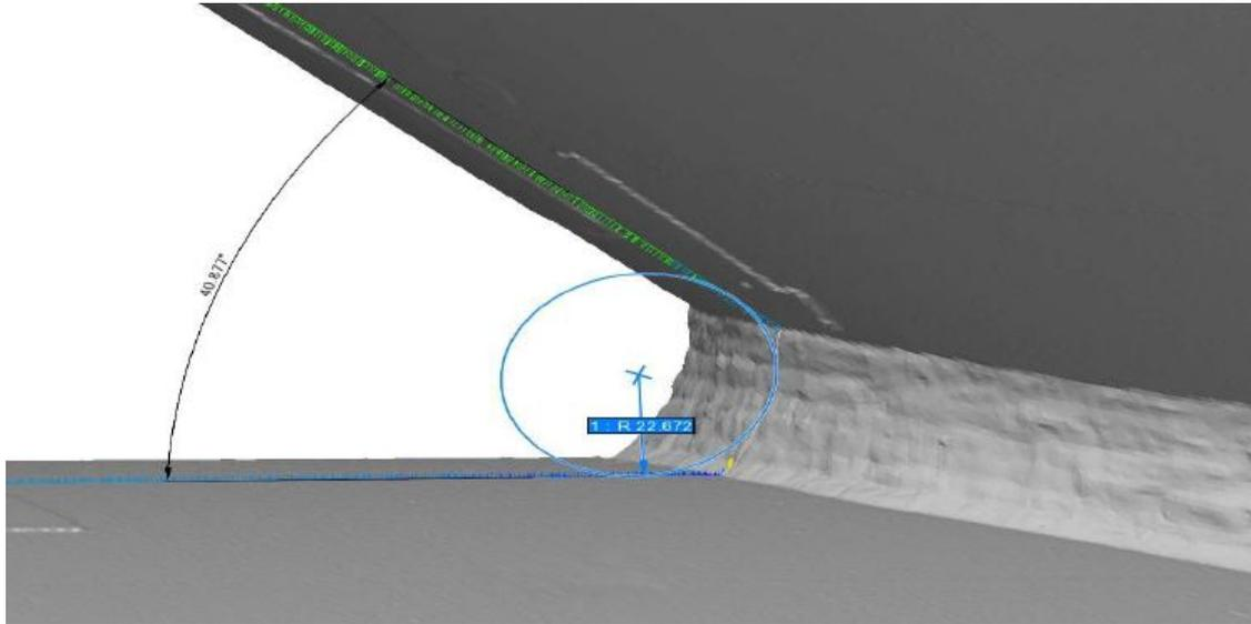
Figure 4: Weld Radius Profile at Acute Node Area to Comply with Standard
