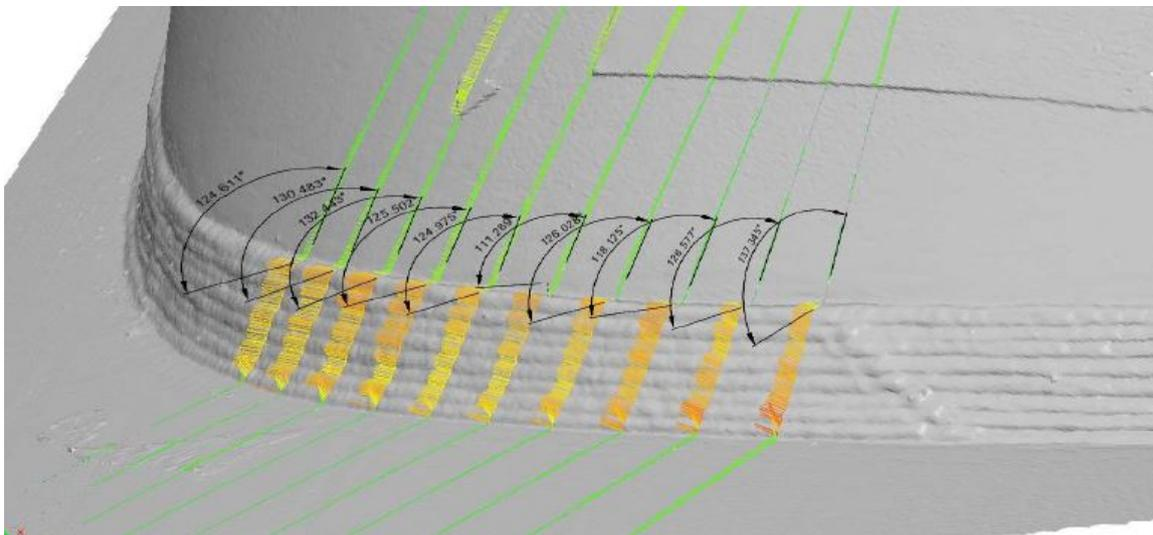
Figure 2: Toe weld angle
