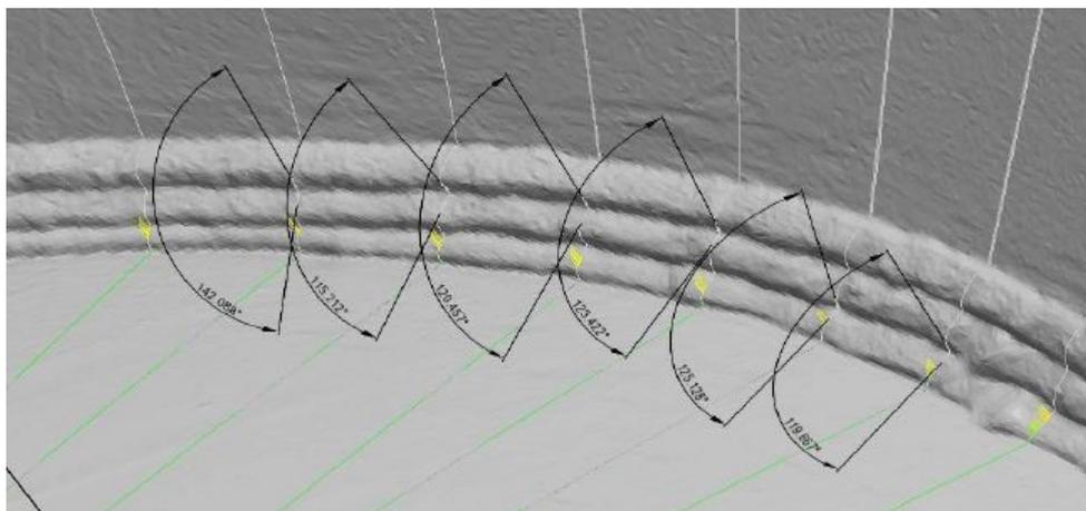
Figure 3: Weld angle between Cap Weld run to check possible Stress Concentration Factors (SCF)
