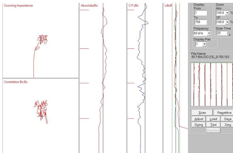
Figure 8: ACFM Change in Permeability/Hardness
