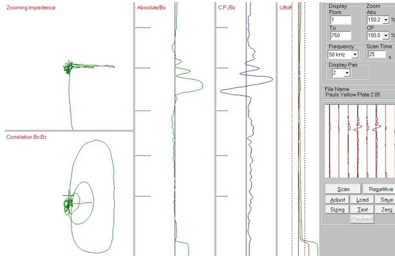
Figure 7: ACFM Crack Indication and Location
