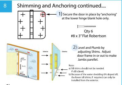
3) Install the remaining anchors in accordance with CSA A440.4 (Figure 7 shown)
