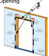
Do not slide the bottom of the door into the opening. (Sliding will damage sealant lines) Position the Door at the bottom on an angle and tilt into place.
