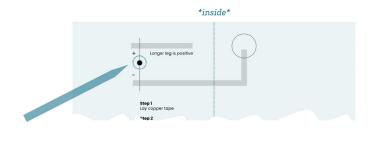
place the LED light through the hole with the legs spread out
