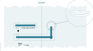
place a piece of the double-sided tape where the battery will be placed
