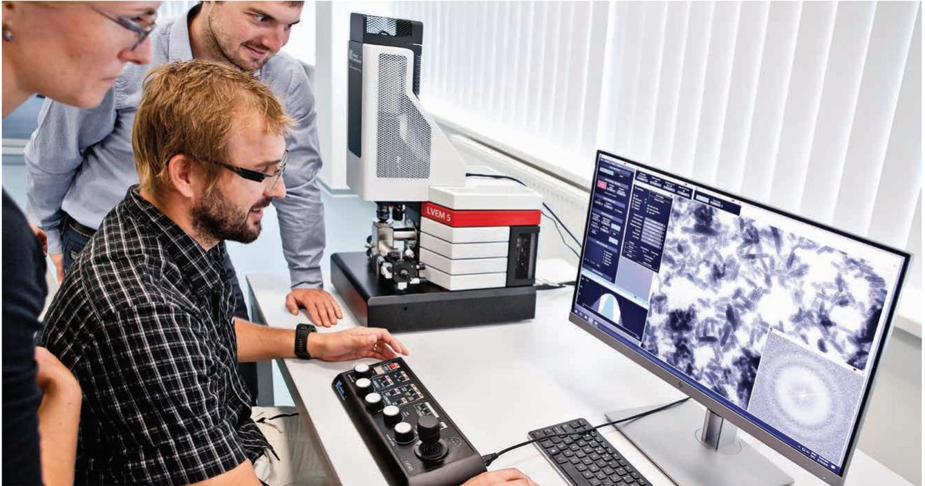
The LTEM 5 seamlessly combines 4 different imaging functionalities into one benchtop instrument, so samples no longer need to be displaced from one microscope to another. Furthermore, switching between imaging modes is easy, with the click of a button the same area of interest of a sample can be imaged in TEM, SEM and STEM modes.
