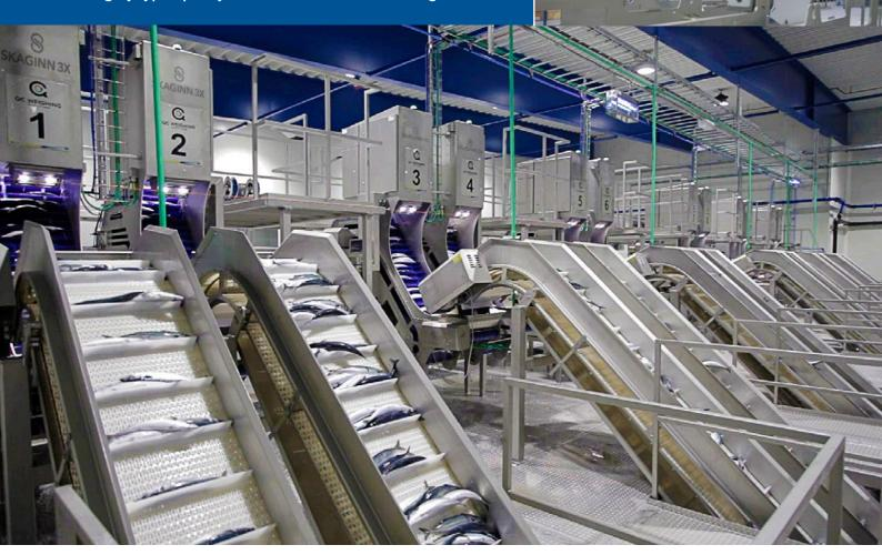
**The QC-Vision Batcher** is a new high speed weigh batcher with automatic quality control system and flow control.
