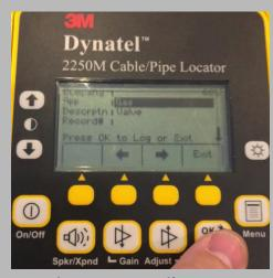
Data is automatically streamed to Orbitas Field.... Have the audio on, so that you can listen for the "Whistle" tone to let you know the marker was read and transmitted to Orbitas Field. The "Description" placed in the marker template, will be read as the feature type. In this case, "VALVE". If you wish to have features set up to match, you must set up a configuration with Tri-Global. Otherwise, data will simply be read and will not be editable once inside of Orbitas Field.
