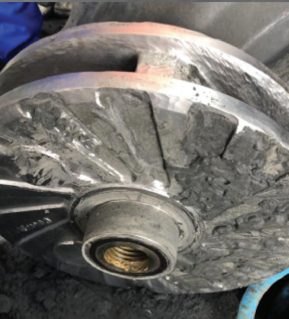
Images above show the Impeller after 12 weeks of running.
