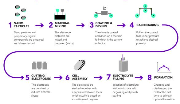
Standard production process allows for use of existing production lines
