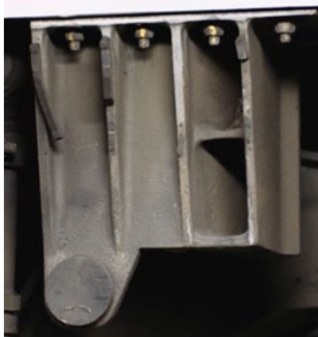
Deutsche Bahn 3D printed, tested, and implemented a secondary roll-stop in half the time of a conventional part.
