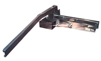
Wynright's Bow Arm Sorter can be used as an integral sortation component in almost any conveyor system. Our high speed induction conveyor strategically gaps and places the product onto the sortation belt conveyor. The Bow Arm Diverter fires to the fully divert position prior to the carton reaching the arm and diverts the product onto a powered or non-powered 45 degree take-away conveyor. This diverter will maintain the orientation of the product from the sortation conveyor through the take-away.
