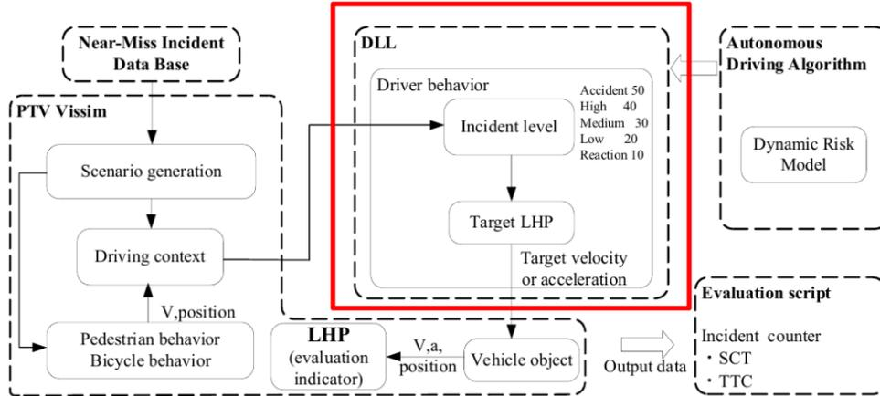
Fig. 4: Integration of new autonomous driving algorithms into the traffic simulation PTV Vissim and evaluation tools
