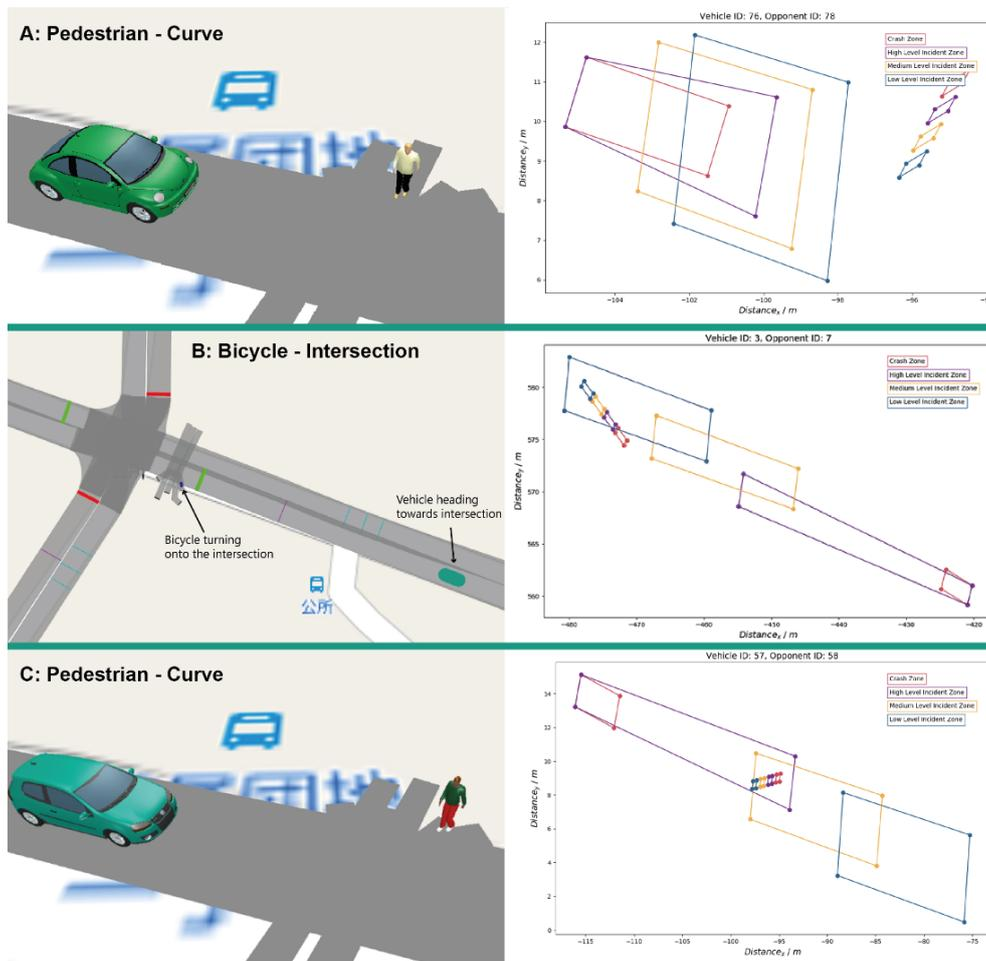
Fig. 7: Examples of critical situations during the simulation with PTV Vissim leading to different incident ratings
