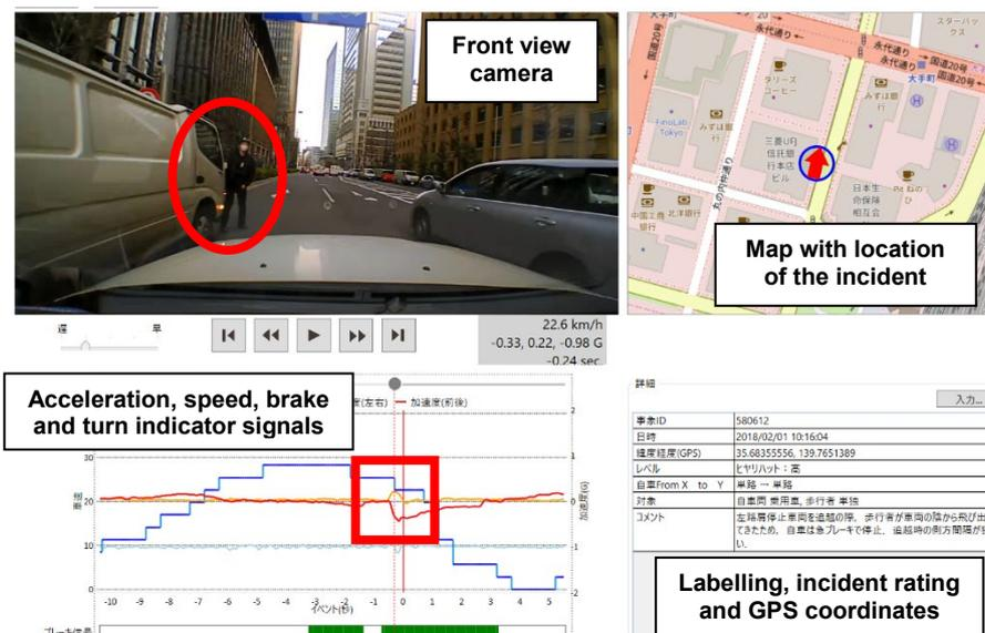
Fig. 1: User interface for manual labelling of incidents in the Near-Miss Incident Data Base
