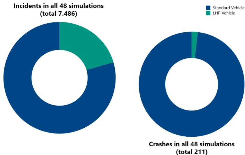
Fig. 9: Comparison of the number of incidents and crashes of the standard vehicle and the LHP vehicle
