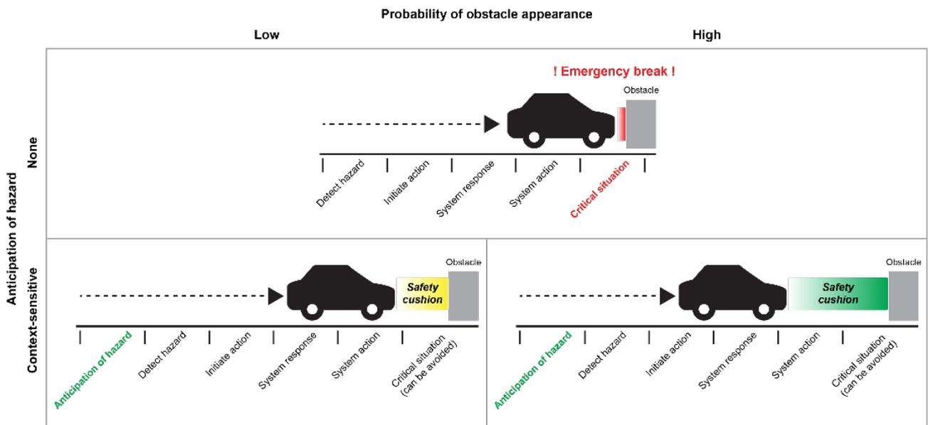
Fig. 3: Safe and comfortable ride by adjusting the Safety Cushion depending on the obstacle appearance probability
