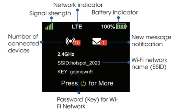
**Note:** Display screen will timeout after 1 minute of inactivity to save power. Press the Power/Navigation button to wake the screen. This default setting can be adjusted in the online WebUI.
