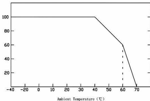
Load carried in accordance with the derating curve, according to the ambient temperature, in order to extend the working life.
