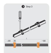
Repeat step 1 & step 2 for the remaining brackets and secure at least 2 locking points for each mounting profile and the equal interval is more recommended.
