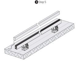
Install the fixture into the mounting profile and leave the front connector and end cap outside of the mounting profile.
