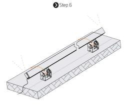
Power on the fixture and rotate the bracket until the mounting profile and fixture are at the desired angle.
