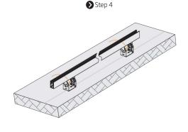
Rotate the bracket back to the upright position. Skip to step 7 for extended lengths (one piece of fixture crossing multiple pieces of mounting profiles).
