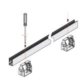
Secure the mounting profile to the rotary locking bracket with screws. (PWM3\*6 - Pan Head Screw, ~3x6mm thread)
