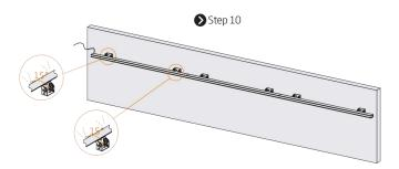
If you need further adjustment after installation, fine tune each rotary locking bracket 15 degrees at a time to avoid excessively twisting the fixture.
