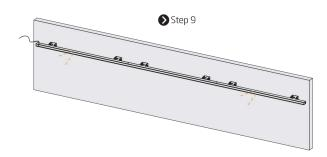
Adjust the rest of the mounting profile to the same angle and then install the remaining coiled fixture orderly.
