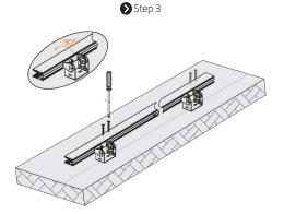
Rotate the bracket to 90 degrees allowing the mounting profile to lay aside. Secure the rotary locking bracket to the mounting surface with screws along the marked line. (KA3.5\*25 - Flat Tip Screw, ~3.5x25mm thread)
