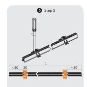
Repeat step 1 & step 2 for the remaining brackets and secure at least 2 locking points for each mounting profile and the equal interval is more recommended.
