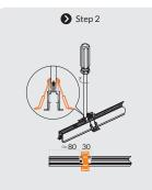
Slide forward ceiling mounting bracket 80mm and fix the screw tightly.
