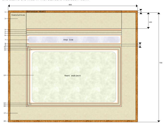
The box design allows for virtually any starting temperature and end temperature over different durations by altering the thickness of insulation.
