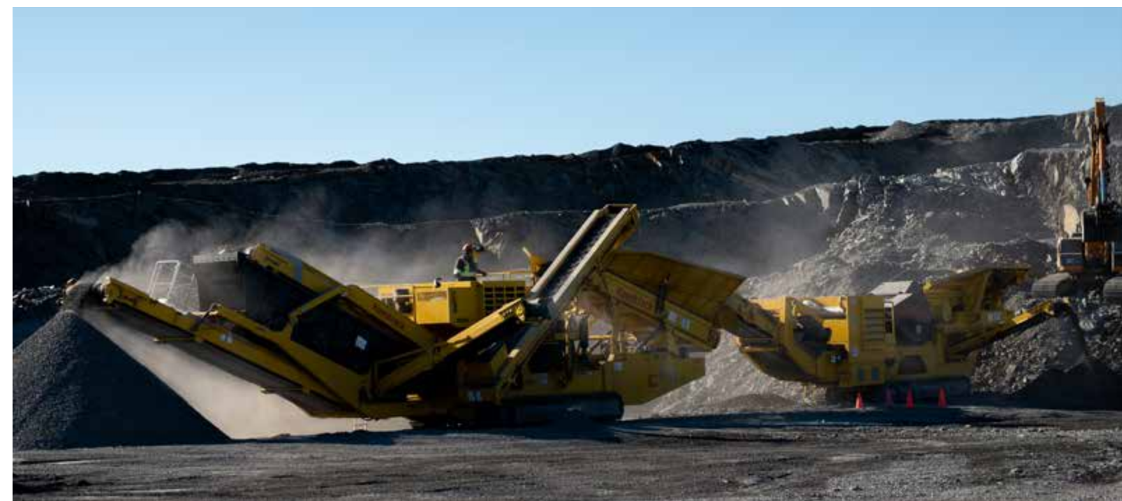
Bottom photo: The Keestrack B4 Jaw Crusher and H4e Cone Crusher processing shale/slate pit material into 20mm basecourse. – Frontline Machinery, all rights reserved by the copyright owner.
