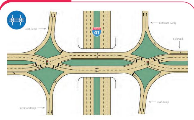
WisDOT is considering the use of a **diverging diamond interchange (DDI)** at highway interchanges across the state including along I-41. This innovative interchange, sometimes called a "double crossover diamond," is designed to gradually direct cars to veer left or right.
