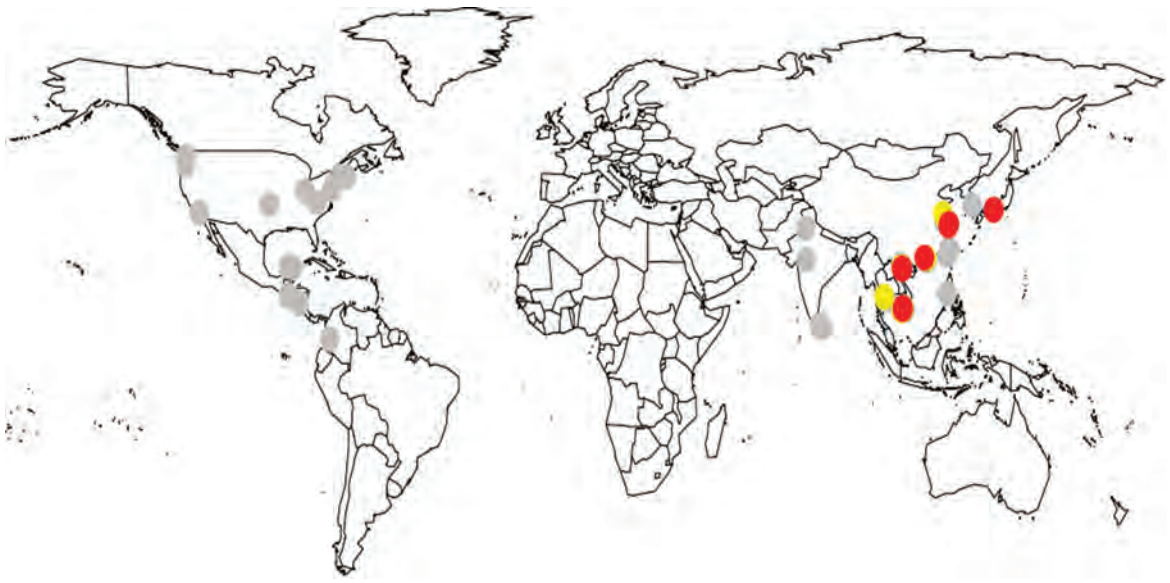
Figure 1. Locations associated with supply chain of a clothing retailer. Shading reflects flood heights associated with 200-year return levels in 2050 based on intermediate future greenhouse gas scenario. Gray shading indicates minimal water heights, yellow indicates water heights up to 3 m, red indicates water heights over 3 m.
