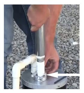
Then, slowly lower the bell end of the top drop pipe into the safety tool (left). Use a channel lock to remove the riser tube and pump head. This allows access to the 3/4" stainless rod.
