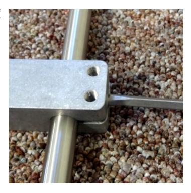
Rotate the Linear Bearing Link Drive Mechanism around the pump head until the holes for the four mounting bolts are aligned.
