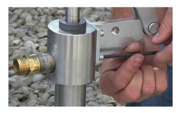
Remove the lever arm bracket and lever (they should still be connected) from the 3/4" stainless rod. The direction you screw is the opposite of normal -- turn clockwise to remove, rather than the normal counterclockwise.
