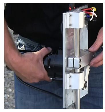
The tolerances are tight between the yoke ID and shaft OD. You MAY need to splay the gap in the yoke slightly, as shown in the photo.
