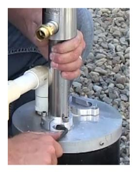
While holding the pump head by the riser tube, seat the safety tool securely in the split flange.
