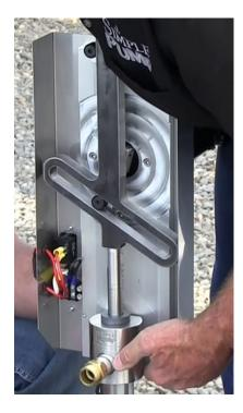
Bring the cam roller (attached to the crank arm) into the cam track part of the yoke (the cam track is the hole in the yoke that is oriented at around 45 degrees), while also positioning the top of the Scotch Yoke (on its grooved side) into the guides at the top of the gear motor mechanism.
