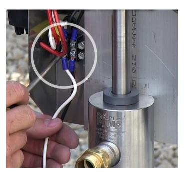
Attach your positive and negative power leads to the terminal block so that the final output rotation is counter-clockwise. This rotation direction will provide a constant tightening torque on the driven cam roller and will prevent the cam roller from walking off of the crank arm.
