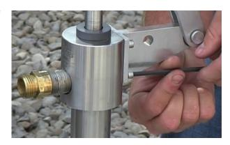
Remove the lever arm bracket and lever (they should still be connected) from the 3/4" stainless rod.
