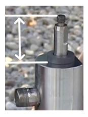
Push the pump rod fully down. The length of the white arrow in the picture should be no higher than 3¾" from the top of the stainless steel rod down to the shoulder (metal top) of the head (left).
