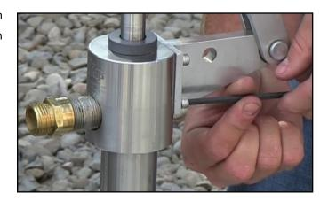
Remove the lever arm bracket and lever (they should still be connected) from the 3/4" stainless rod (right).
