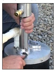
While holding the pump head by the riser tube, seat the safety tool securely on the split flange.
