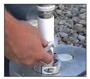
Then lower the riser tube so that at least 6 inches of riser tube are below the split flange on the cap.
