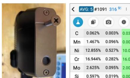
**Fig. 3.** SciAps Z-902 Carbon analysis of 1" s/160 A106 pipe nipple for HF Alkylation service
