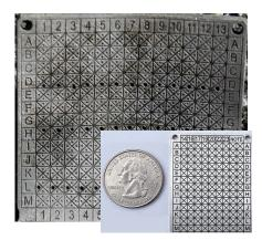
To protect bitcoin backup seeds, metal storage devices have been developed. In the background you can see one such device after it was exposed to stress tests involving heat, corrosion, and crushing. For more, see Jameson Lopp's excellent tests and reviews in this area.
